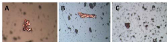
Fig. 6 Ferrograms of electric arc test samples. A: Copper sphere. B: Copper piece. C: Red oxides
