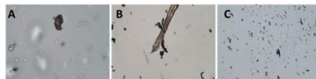
Fig. 4 Ferrograms of test II samples. A and B: Copper. C: Dark particles
