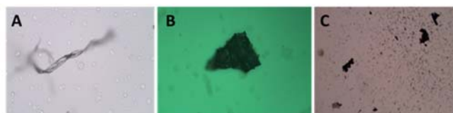
Fig. 3 Ferrograms of test I samples. A: fiber. B: Carbonized paper. C: Dark particles
