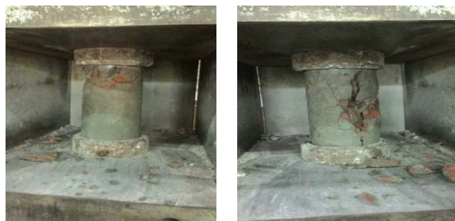
Fig. 10 Failure pattern during crushing strength test (7 days)
