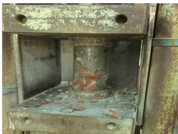
Fig. 9 Failure pattern during compressive strength test (28 days)
