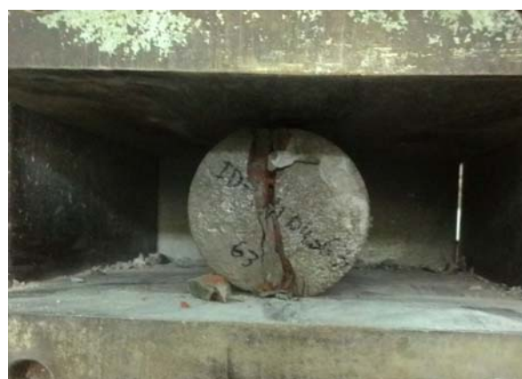
Fig. 11 Failure pattern during tensile strength test (7 days)
