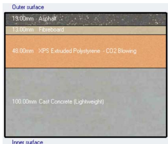
Fig. 5 Roof with xps polystyrene insulation
