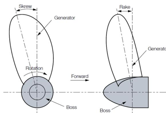
Fig. 1 Rake and skew angle
