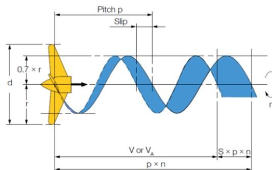
Fig. 3 Different characteristic of the propeller
