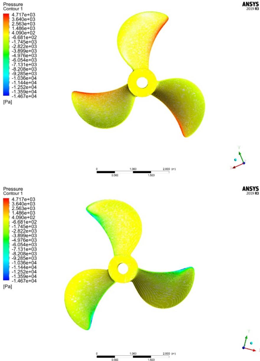
Fig. 4 Pressure distribution on propeller
