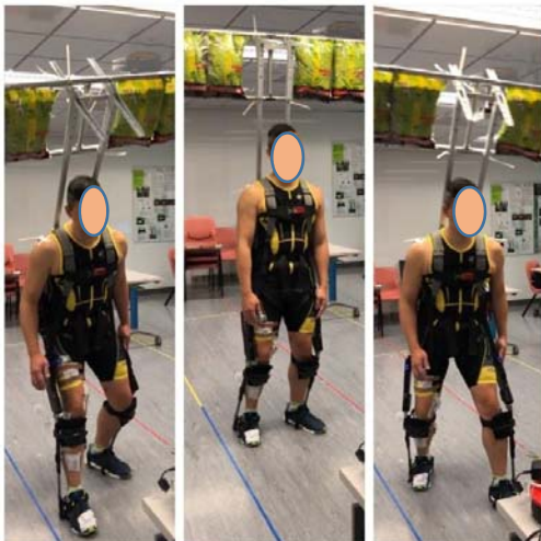
Fig. 7 Participants are required to walk/slide 6 left + 6 right steps alternately forth and back, totally 4 cycles, 48 gaits, total 4 x (20 +/- 4 sec.)
