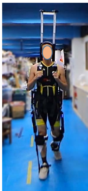
Fig. 2 SuitX system, total handling weight is 22.68 kg. (BackX - Model AC hardware weighs 3.4 kg and LegX weight 6.2 kg, Exoskeleton Harness that weighs 1.1 kg + an external weight 11.98 kg)
