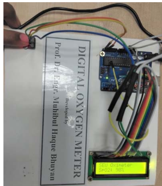
Fig. 6 Implemented digital oxygen saturation level measurement system on a breadboard
