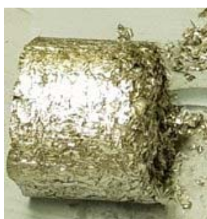
Fig. 5 As received briquette from Renishaw.
