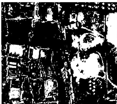
Fig. 15 Change detection from the QuickBird image to the WorldView image of "Scene 1" after 13 years have passed: White = change, Black = no change [19]
