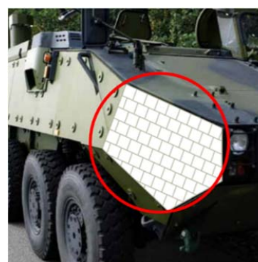
Fig. 2 Ceramic composite armor used for military vehicles [10]
