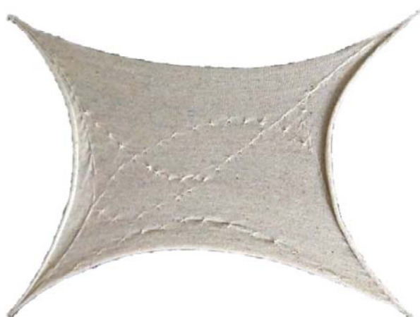
Fig. 4 The resulting flat knit before being stretched into shape
