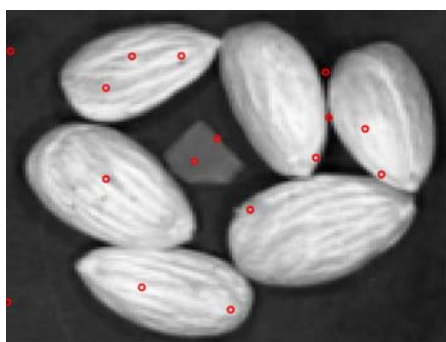
Fig. 1 Localization of endmembers in image 1. Endmembers were found using SG algorithm. This image contains plastic 1 and almond seeds, with a background
