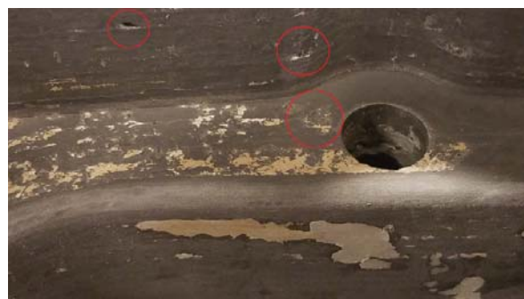
Fig. 10 Chipping defects of the mold surface
