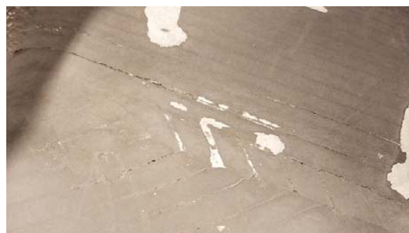
Fig. 11 Cracking defects of the mold surface
