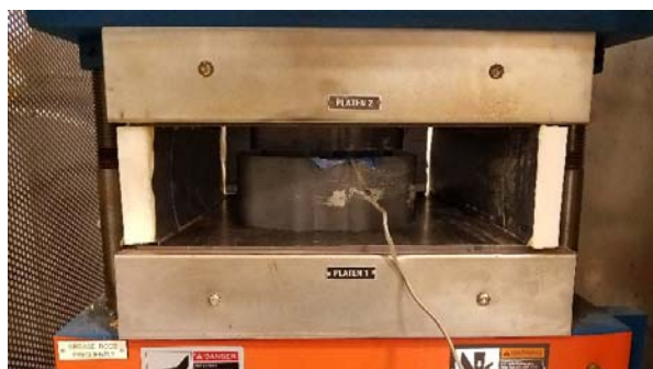
Fig. 8 Mold assembly loaded in heated press
