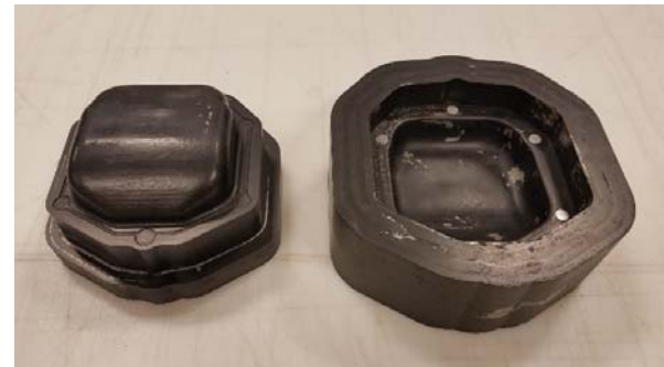
Fig. 5 Completed 3D printed composite compression mold
