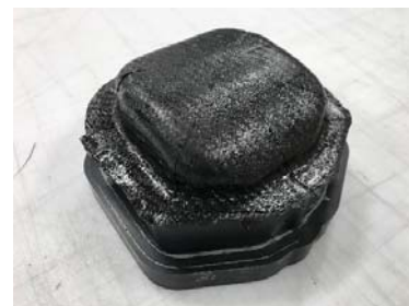
Fig. 6 Carbon fiber valve cover layup
