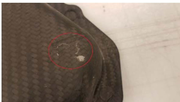
Fig. 15 Carbon fiber valve cover defects
