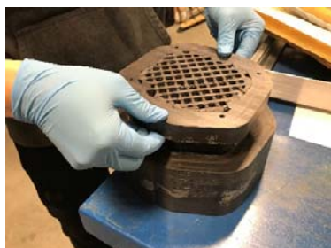
Fig. 7 Completed compression mold assembly
