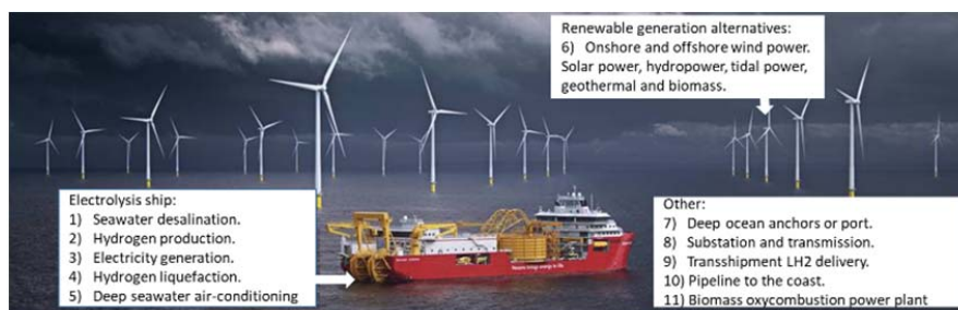
Fig. 1 Electrolysis ship components
