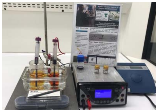
Fig. 2 The controlled-potential organic electrosynthesis cell design
