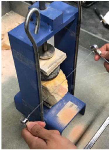
Fig. 5 Uncemented sandstone trimming process
