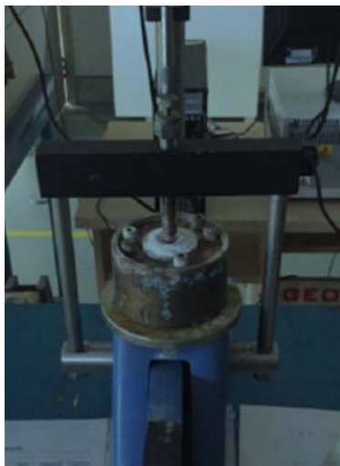
Fig. 6 Oedometer test set up.
