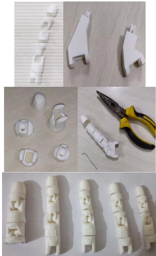
Fig. 7 Different parts of fingers and the assembled finger
