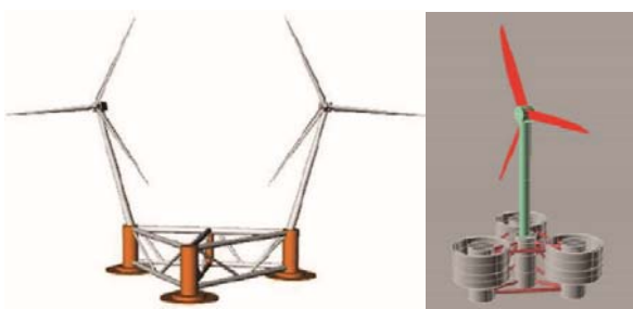
(a) twin turbine structure [49] (b) single turbine tripod [50]
