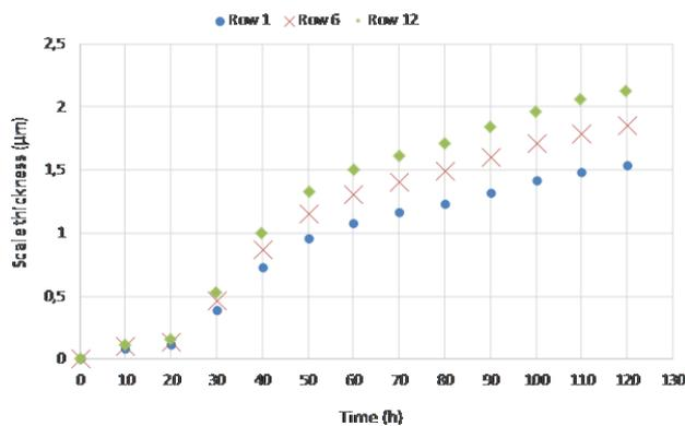
Fig. 3 Variation of the scale thickness in different bundles of the evaporator; working conditions in Table I
