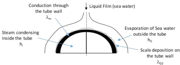
Fig. 2 Heat and mass transfer in the FFHTE
