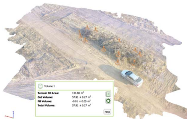
Fig. 7 Models of test area from UAV during test trials in Israel (April 2017): using images from DJI Mavic Pro
