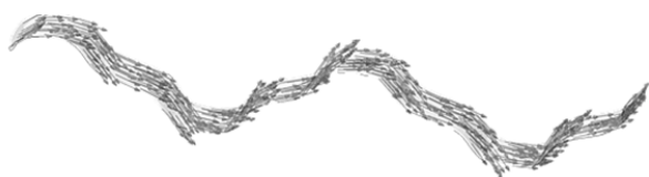
Fig. 6 Material orientations on a binder yarn
