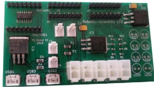
Fig. 6 Electronic board designed to provide different voltages
