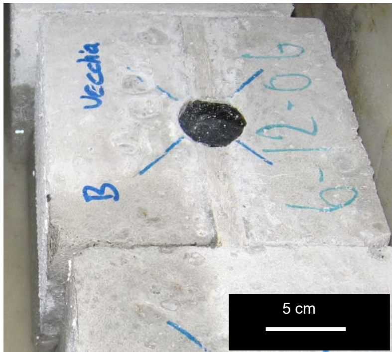
Fig. 1 Concrete cube of 150 mm length with the central cylindrical cavity filled with the resin
