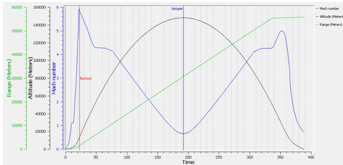
Fig. 12 Variation of the altitude, fall range and Mach number of the vehicle throughout the flight time [20]
