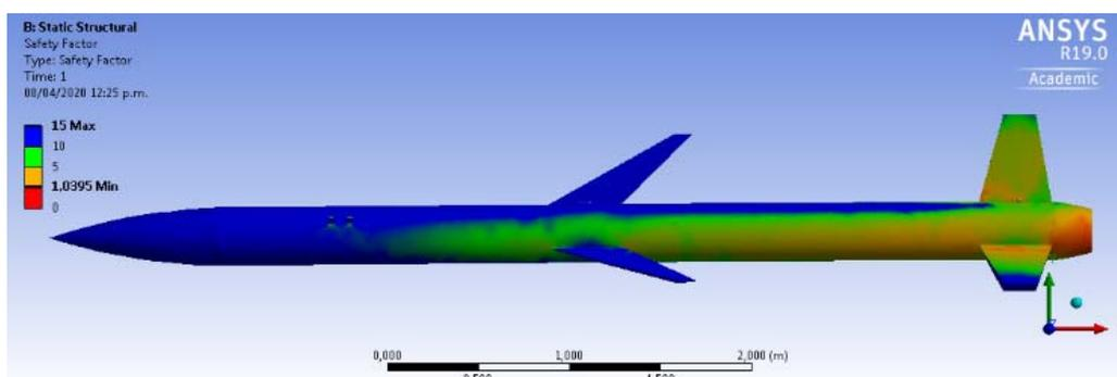
Fig. 18 Safety factor of the rocket at Mach 6
