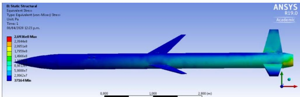
Fig. 16 Equivalent stress of the rocket at Mach 6
