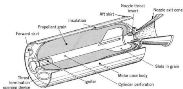
Fig. 1 Representation of a solid fuel engine [9]
