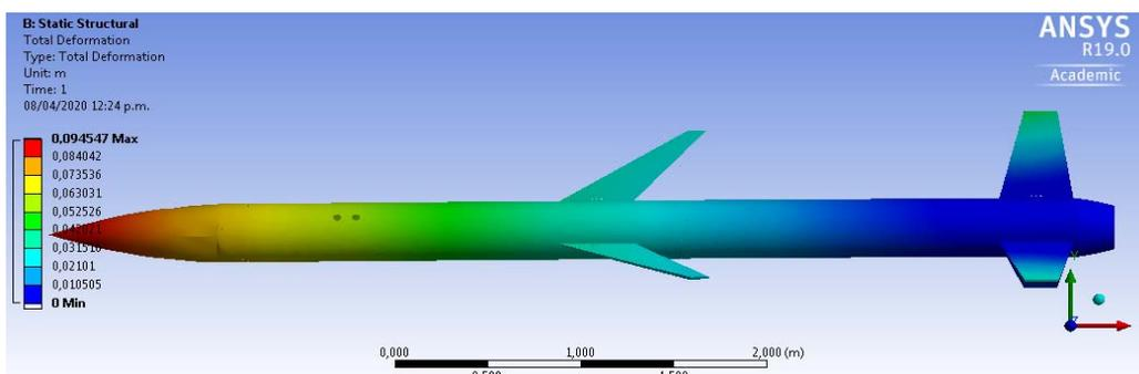
Fig. 17 Total deformation of the rocket at Mach 6
