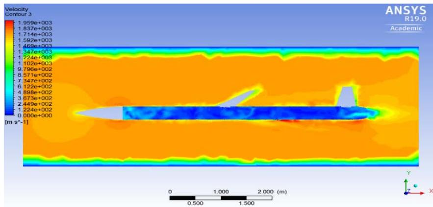
Fig. 14 Velocity contour of the rocket at Mach 6
