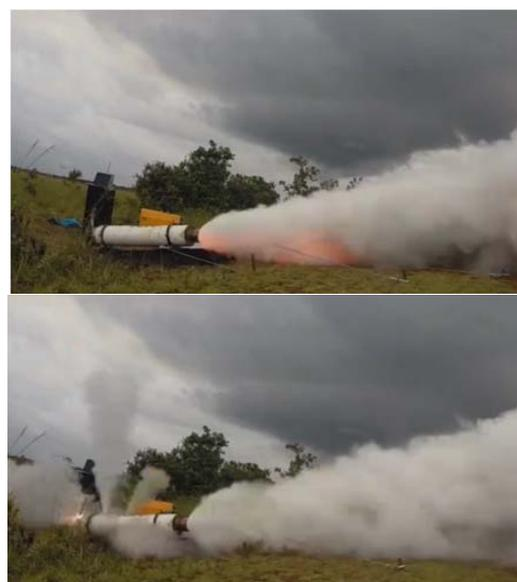
Fig. 3 Illapa 1 engine test and failure [10]
