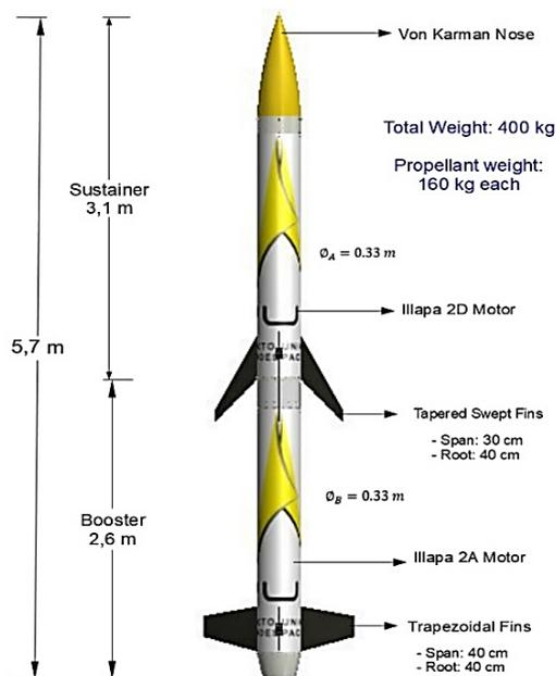
Fig. 11 Dimensions and main characteristics of the rocket
