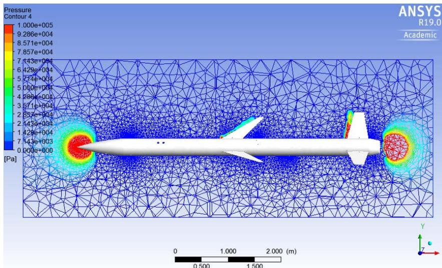
Fig. 15 Pressure contour of the rocket at Mach 6
