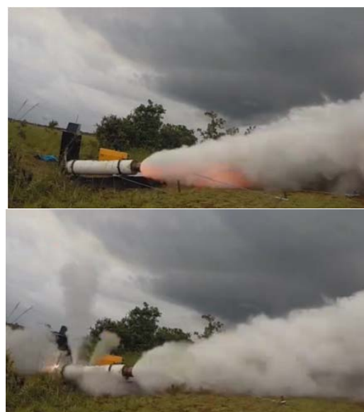
Fig. 3 Illapa 1 engine test and failure [10]
