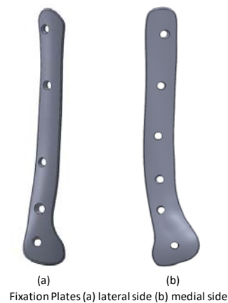
Fig. 3 Customized implant designed for fractured bone
