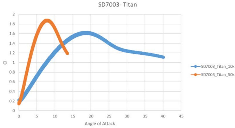
Fig. 11 C_l vs \alpha for SD7003 on Titan at Re = 10000 and Re = 50000 with k = 0.25 rad/s
