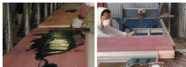
(a) Gluing sandwich panels (b) Cutting of sandwich beams
