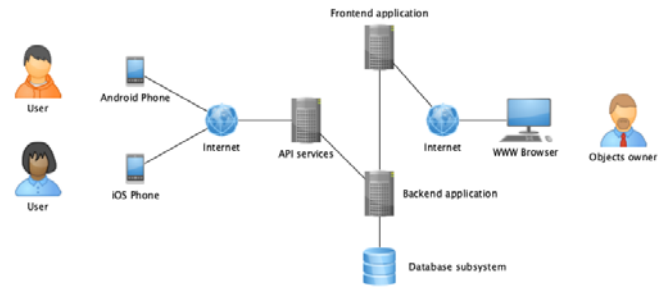
Fig. 5 Overview of the DotAuth authentication system architecture
