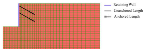
Fig. 16 Geometry of dimensionless excavation model analyzed in evaluating of allowable horizontal displacement
