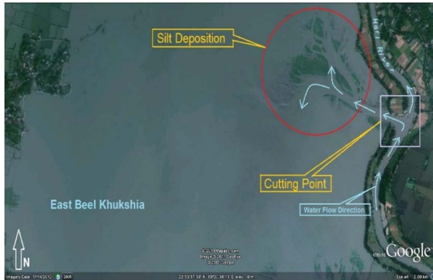
Fig. 4 Cutting Point and Silt Deposition point of Beel Khukshia
