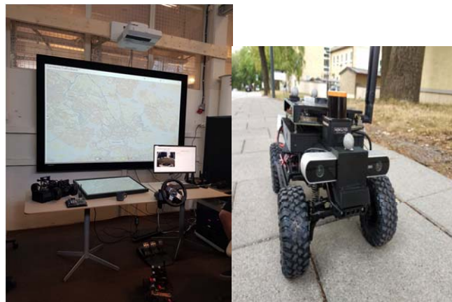
Fig. 4 Prototype of remote control station and scale-down AV
