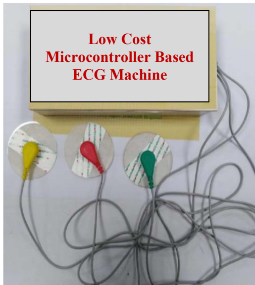
Fig. 5 Complete set-up of the designed ECG machine
