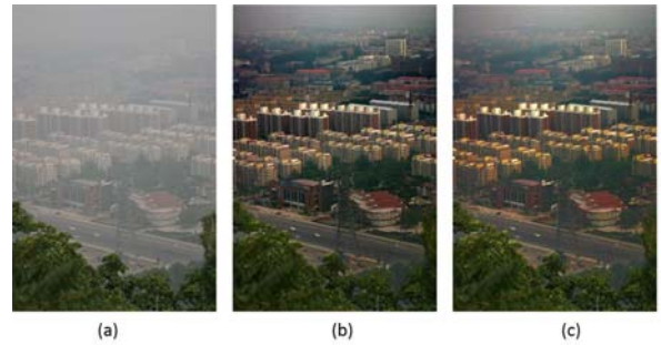
Fig. 12 Canon - Contrast and Color Fidelity Comparison (a) Hazy image (b) Traditional DCP (c) Proposed method
