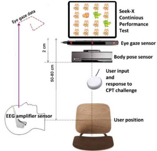
Fig. 2 The multimodal multisensor experimental platform with the eye gaze, body pose, EEG sensor and the CPT
