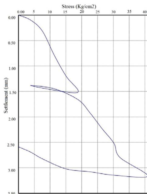
Fig. 4 Typical results of static loading test
