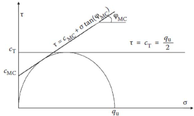
Fig. 1 Two proposed failure models for JG columns
