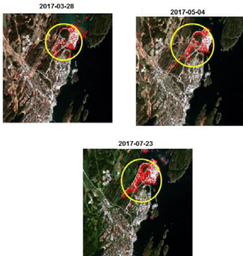
Fig. 7 The changed pixels shown as red squares in three different dates of Sentinel-2 images as a result of GLRT test
