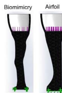
Fig. 13 Loading conditions for prosthesis
