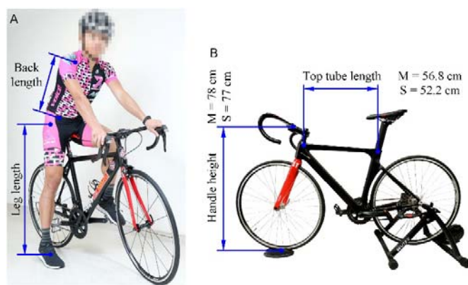
Fig. 1 Schematic diagrams of (A) the measured leg and back lengths of cyclist riding the bicycle, and (B) the configurations of small (S) and medium (M) size bike frame employed in this study
