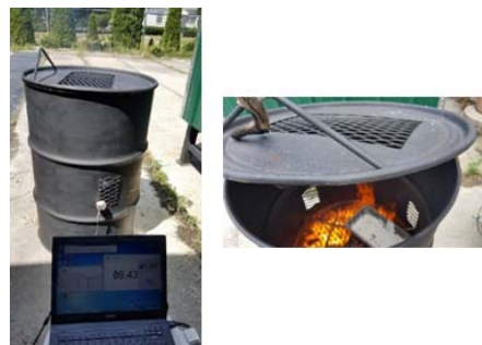
Fig. 3 Indigenous (barrel) furnace used for activation of clay through combustion of wood
