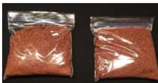
Fig. 2 Red clay used as aluminosilicate precursor in synthesizing the indigenous binder
