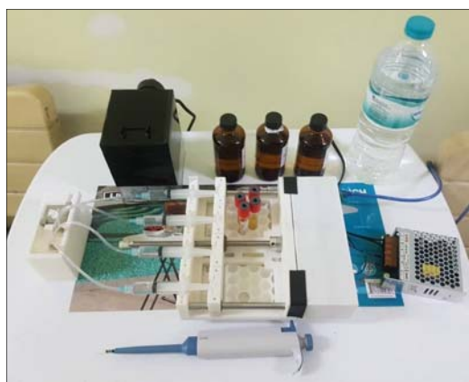
Fig. 3 RPHPLC Microfluidics System Hardware Setup
