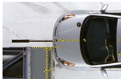
Fig. 1 Moderate Overlap Frontal Test Configuration
