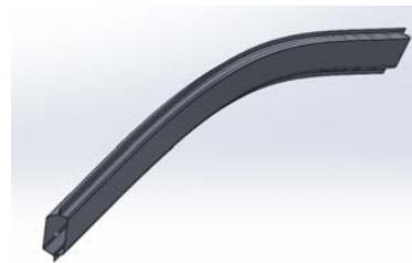
Fig. 9 CAD Model of 2012 Camry A-Pillar
