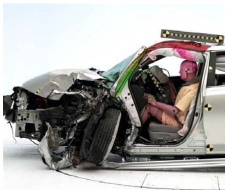
Fig. 15 Overlay of 2012 Camry A-Pillar Simulation on Actual Crash Photo
