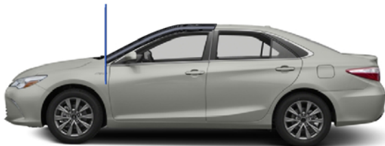
Fig. 12 CAD Modeled A-Pillar Overlay of 2015 Camry
