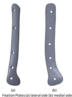
Fig. 3 Customized implant designed for fractured bone
