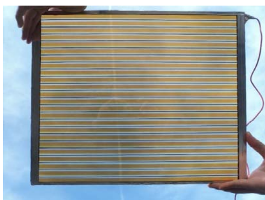
Fig. 2 A highly transparent 50x50 cm 2 DSSC module with 21 serially connected individual solar stripes
