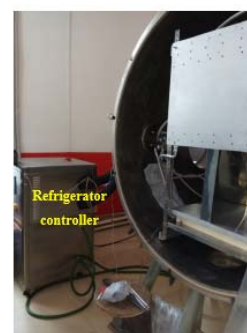
Fig. 24 Adjust the cooling plates and refrigerator temperature
