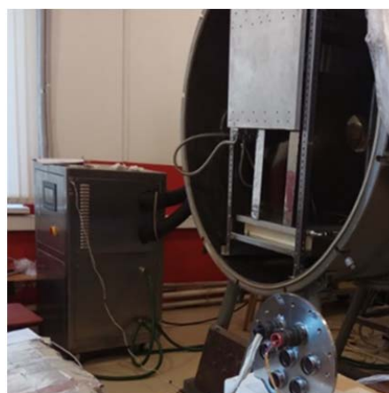
Fig. 14 Cooling system for the MVC
