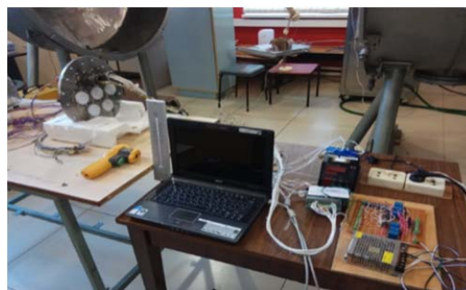
Fig. 28 Connection of the computer with a data acquisition system and onboard control unit
