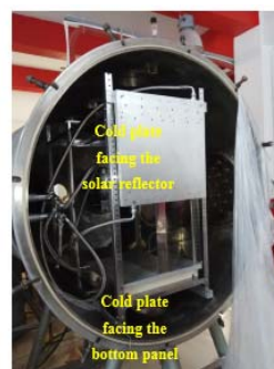
Fig. 24 Adjust the cooling plates and refrigerator temperature
