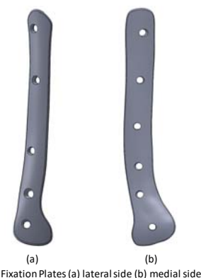
Fig. 3 Customized implant designed for fractured bone
