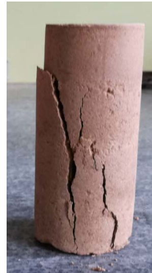
Fig. 13 Specimen failed on unconfined compression strength test
