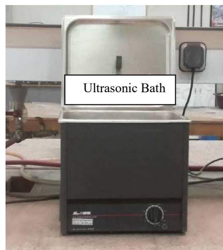
Fig. 2 Ultrasonic bath apparatus
