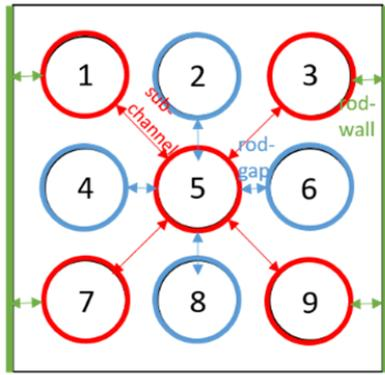
Fig. 2 Cross-sectional arrangements of conductivity probes in the rod bundle test section
