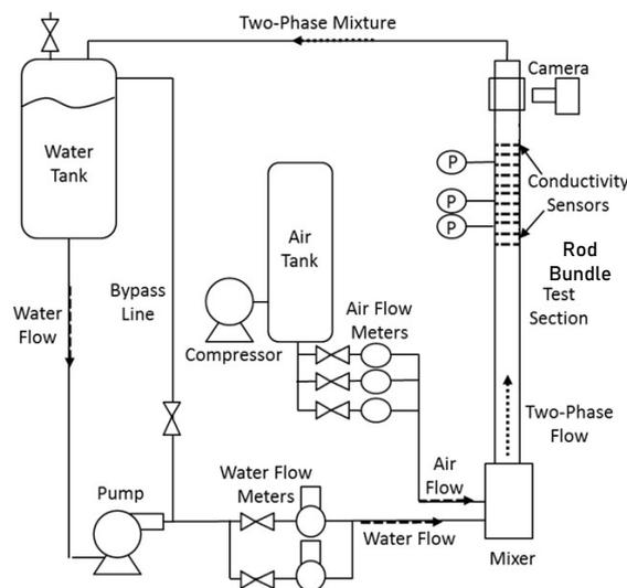
Fig. 1 Schematic of 3×3 rod bundle test facility
