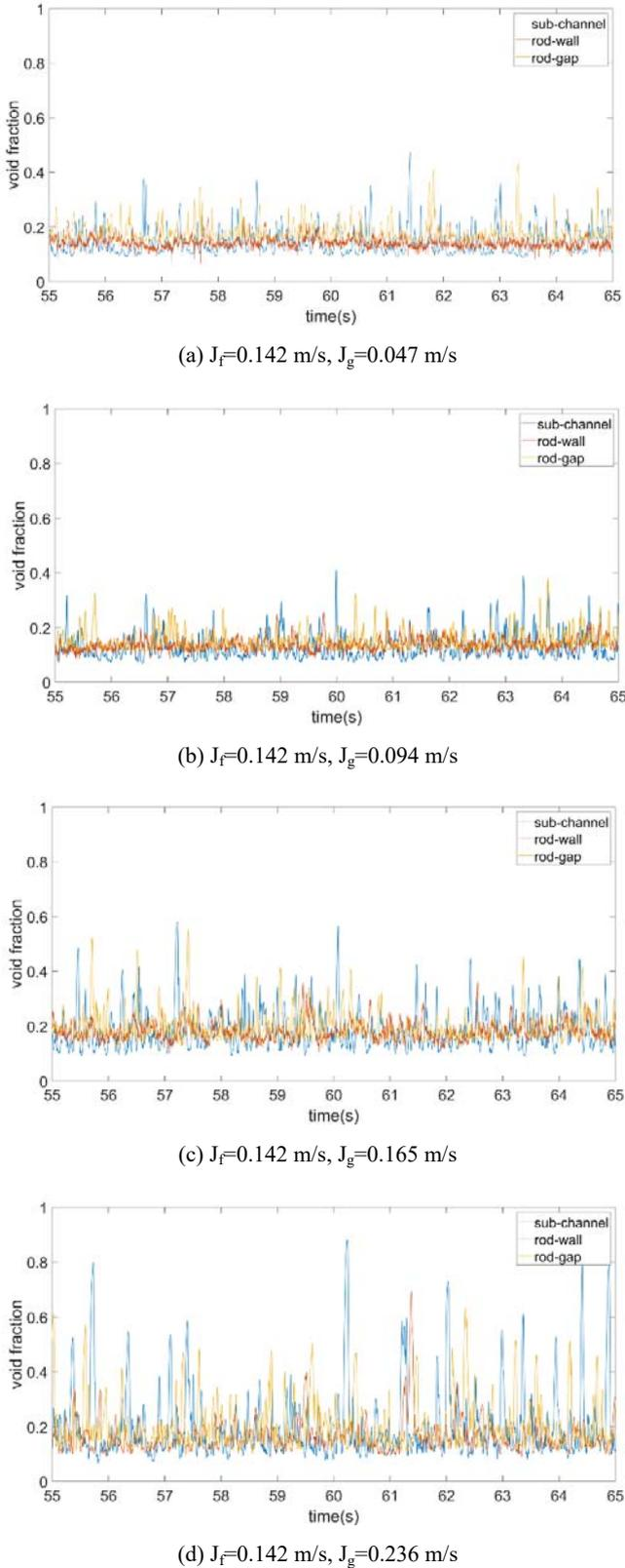
Fig. 4 Void fraction signals under various test conditions
