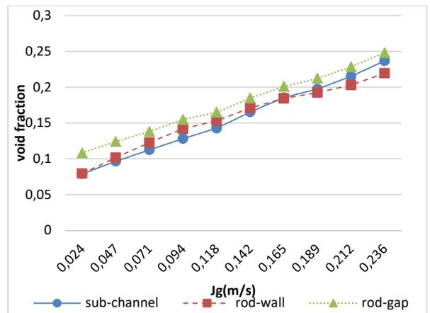
Fig. 5 Averaged void fraction under various test conditions
