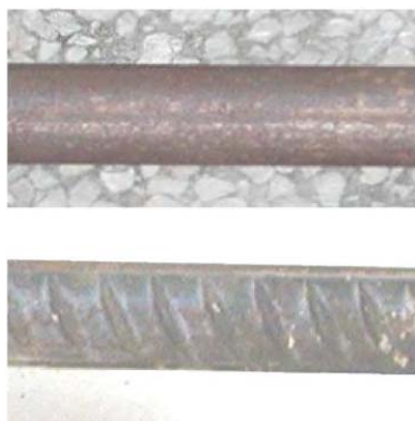
Fig. 3 Bars used as reinforcement [16]
