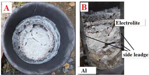
Fig. 4 Cell after cooling: A is a top view; B - cross section
