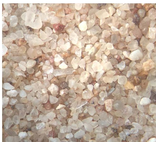
Fig. 1 Optical microscope image of the Firouzkouh sand
