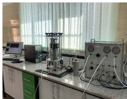
Fig. 3 Resonant column device
